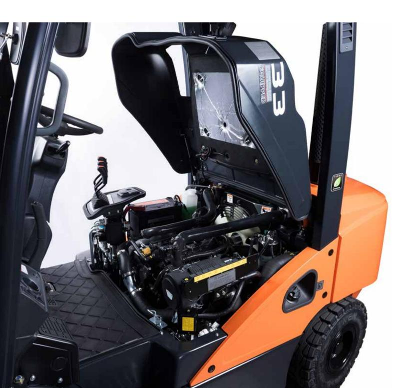
All our powerful diesel and LPG engines are compliant to the current regulations for reduced emissions. These in-line, 4-cylinder, water cooled, overhead valve engines provide high torque at low engine speeds for applications requiring ramp loading and unloading, fast lift speeds, or heavy hydraulic flow requirements.
