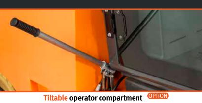
With the tiltable cabin, all main components below the cabin are easy-toaccess which makes the service handier.
