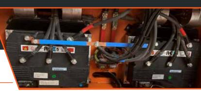
Easy access controller The IP65 rated controller is very reliable, well proven in tough applications and easy-to-access.
