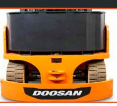
**Battery change system** Thanks to detachable backplate, the battery change for multiple shifts is easier.
