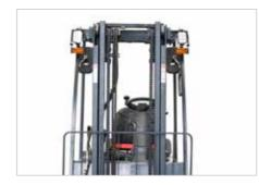
Neatly arranged hydraulic hoses and chains provide clear front visibility through the wide view mast.
